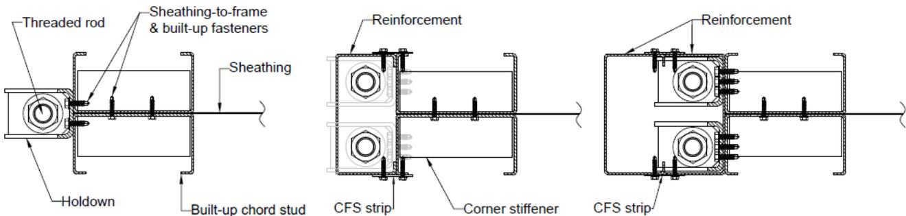
Figure 3. Left to right : no reinforcement, R2, and R3 reinforcement schemes for the chord stud members
