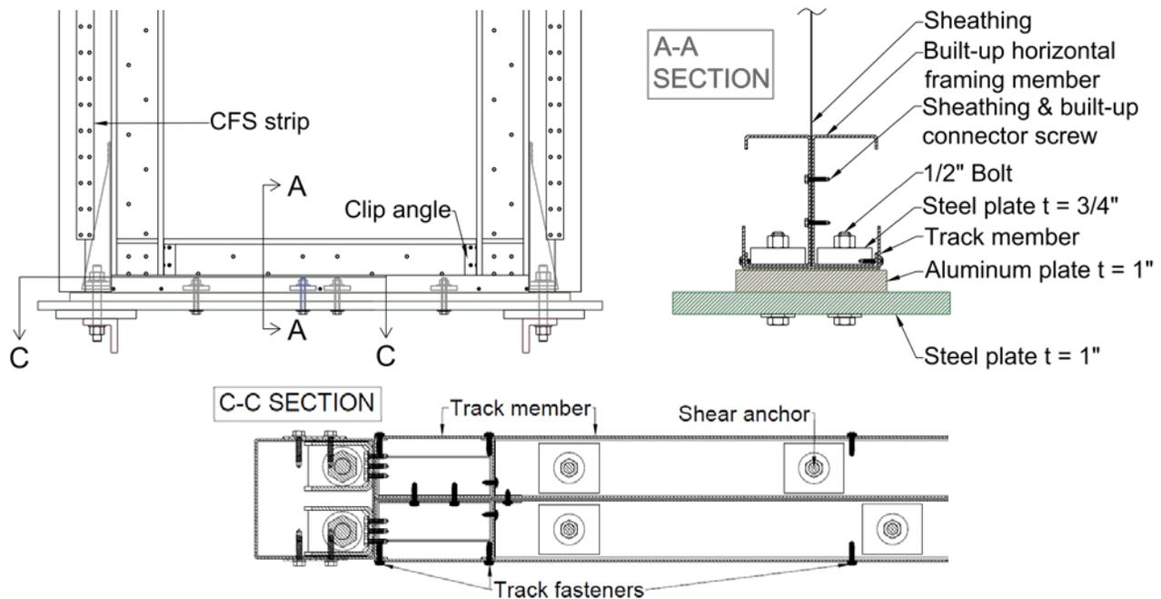
Figure 4. Detailing of centre-sheathed shear wall
