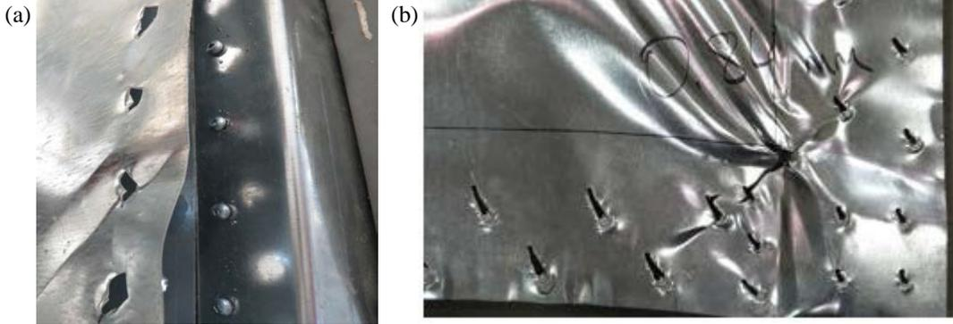
Figure 2. (a) Bearing of exterior sheathing resulting in pullover, (b) bearing of interior confined sheathing (Santos [4])
