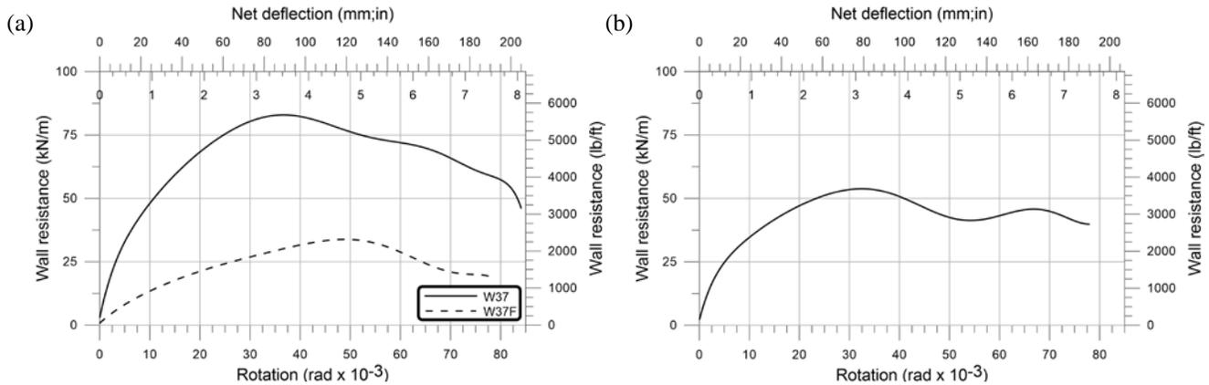
Figure 10. W37 force vs. deformation : (a) full wall and frame-only, (b) Difference between the two backbone curves
