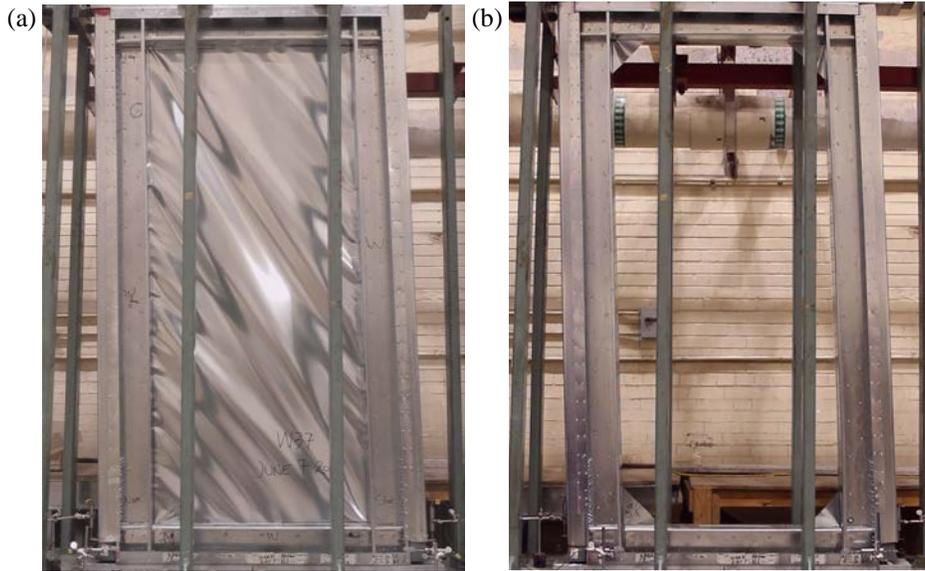
Figure 6. Tension field during testing : (a) Test specimen W35 (b) Test specimen W35F
