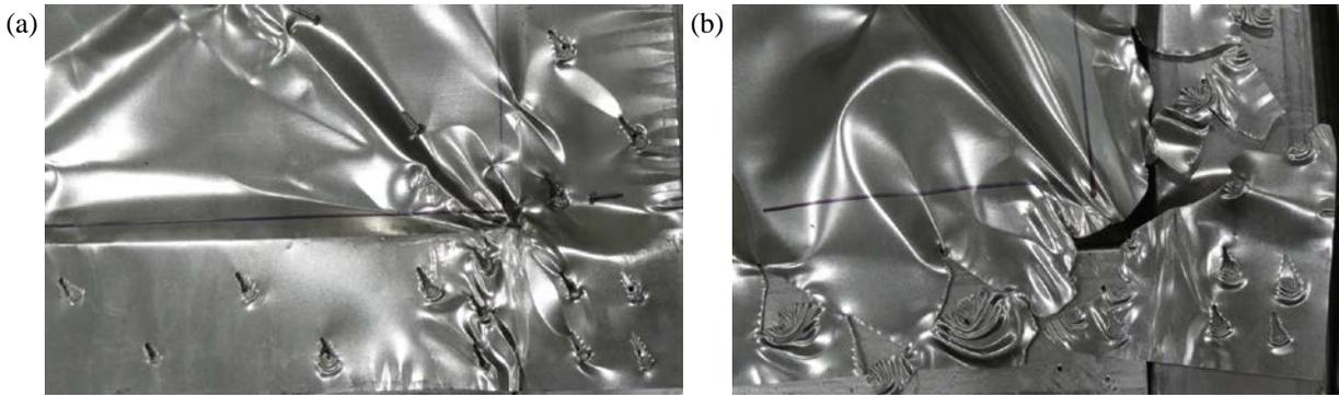
Figure 7. Bearing damage : (a) Specimen W36, (b) Specimen W37 with torn corner due to extensive drift demand
